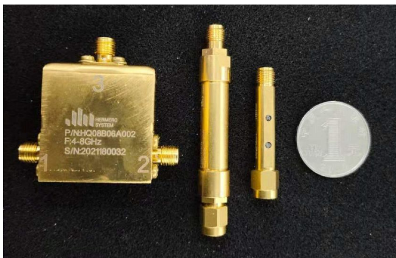
Figure S3, a photo of a cryo-circulator, a LP filter and an IR filter (from left to right ), they are all from Hermetic Inc , China. A coin of one Chinese Yuan is used as a reference of size.
